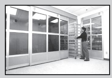
Electronic instrumentation is tested at a constant 131° F prior to acceptance and shipment to the customer.
