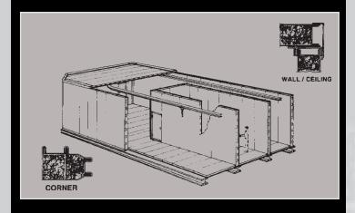
Durable metal clad composite panels are factory fabricated and finished. These are packed with a high density mineral fiber for maximum thermal insulation and noise absorption. A unique slot in the framing members provides for minimum heat transfer to the enclosure exterior. A complete line of trim and accessories is available.
