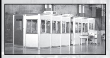
Aircraft maintenance is monitored on hanger floor. Self-contained quality assurance pods are forkliftable and positioned adjacent to tasks.
