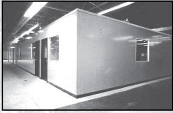
Insulated steel faced panels with baked enamel finish are assembled without the use of exposed joining hardware to provide a clean contemporary surface.
